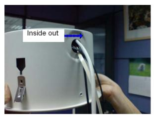
6. Take away 3pcs screws inside the accessory box. Use the screws to fix the inner cover and outer cover.
